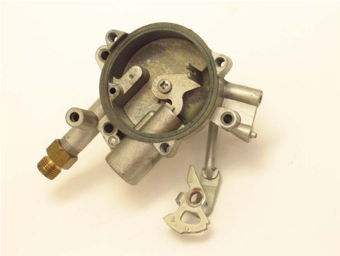
8 The automatic choke assembly as it stands as a separate bolt-on assembly.
